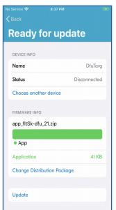
After the transfer has completed, the altimeter will automatically restart into the new firmware and can be connected to the FlightSketch app as normal. The update process is complete.
