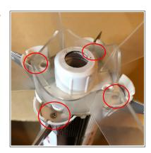
2) Next glue the end centering ring to the motor mount tube. The end of the ring with the 18mm step down should be exposed. The flat surface of the ring should be flush with the end of the tube.
