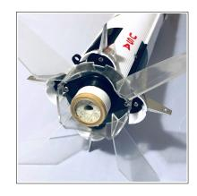
8) To balance, press the included 2 squares of clay into the ring at the top of the main body tube. The CG ready to fly should match the original CG with the C6-3 motor installed.
