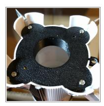
4) Insert the motor mount tube and ensure the adapter ring is seated in the recess in the forward airframe plate.
