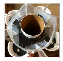
7) Secure the assembly with the provided machine screws. There are 2-56 nuts press fit into the back of the thrust plate.
